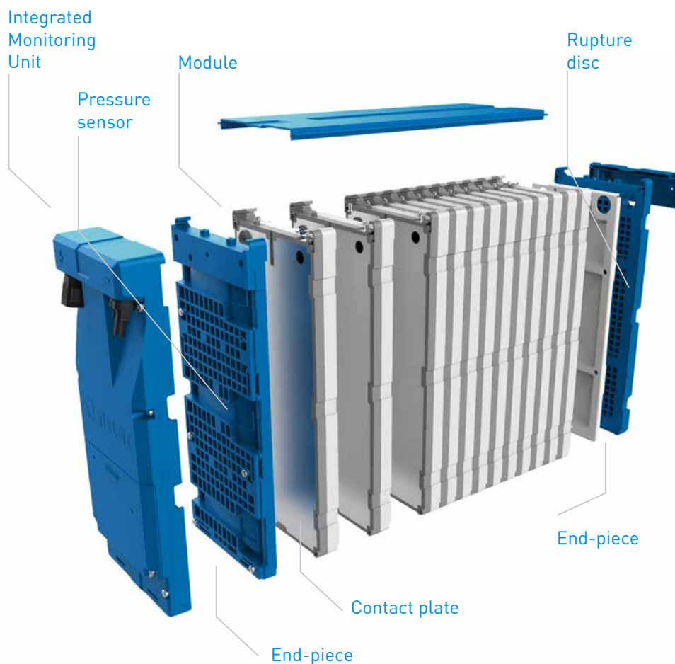
Figure 4. Battery pack expanded view.
