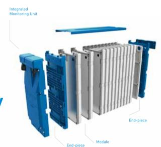
Typically, each battery pack contains between 8-12 modules (12V per module). In turn, every module contains 10 battery cells. Nilar battery packs can deliver high discharge power and accept high charge power. At low cycle duty, more charge and discharge power are available, depending on the battery system and application. Battery packs are designed to be used in systems with a maximum battery voltage up to 800 VDC.
