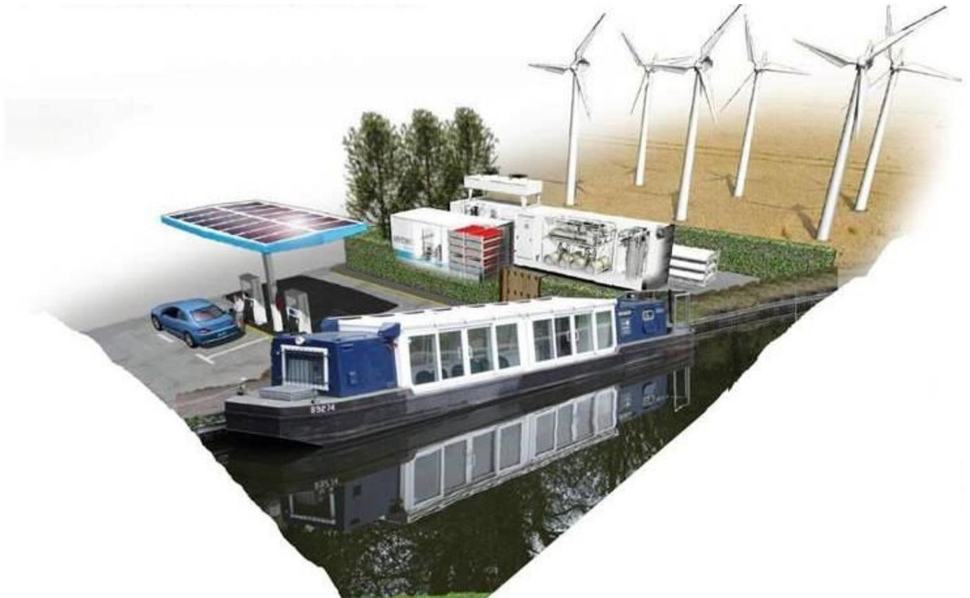
*Nilar has collaborated with the University of Birmingham to convert a British Waterways maintenance craft into a hybrid canal boat for the future. The standard diesel engine of the boat has been replaced by an all-electric propulsion system with a hydrogen store that eliminates atmospheric, water and noise pollution – paving the way for more efficient and environmental transportation. Nilar’s NiMH technology played a vital role in the success of the project.*
